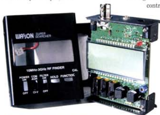
Taking off the case, reveals a single uncomplicated looking board and a large display.
