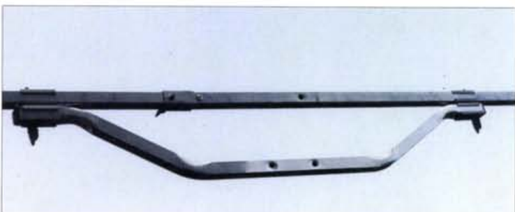
Fig. 7: An alternative support and bracer bar idea to be tried out on the VUH1 antenna, allowing a more central mounting point to be achieved.
