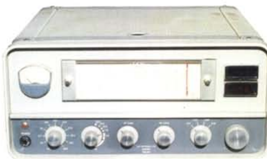
The KW Electronics KW201 double conversion receiver, the indicators on the top right show either upper sideband (u.s.b.) or lower sideband (l.s.b.) is selected. The main tuning knob is on the lower right.
