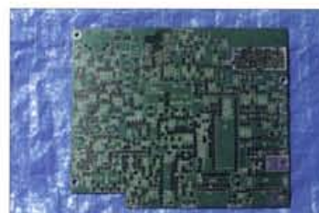
Fig. 3: Above and below, illustrating both sides of the high quality main printed circuit board (with through hole plated interconnections) and component overlay printing.
