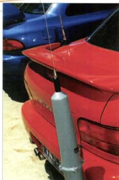
Fig. 3: The Barrett 510 mounted on the back of Chris VK3CE's Subaru WRX (see text).
