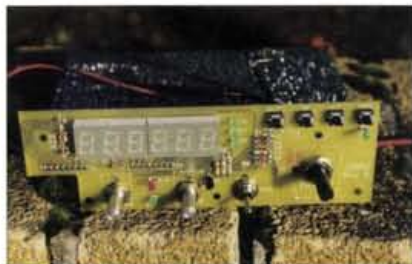
Fig. 5: Main front panel display unit assembled (see text).
