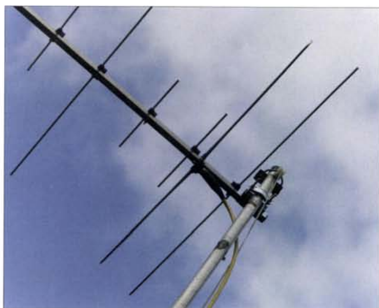
Fig. 6: More details of the feed-point and mounting arrangements for the VUH1 antenna.
