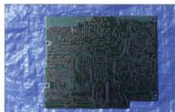
Fig. 3: Above and below, illustrating both sides of the high quality main printed circuit board (with through hole plated interconnections) and component overlay printing.
